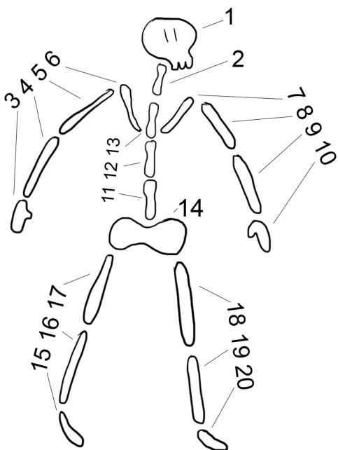
The computer needs to take care of all these skeletal bones and skinning of the mesh each frame of the game. Furthermore each point on the mesh, called a vertex, can be weighted onto more than one bone, which takes even more time to process. So there is a good reason to take it down a notch. Maybe not on the main character, but with crowds it is an absolute necessity.
